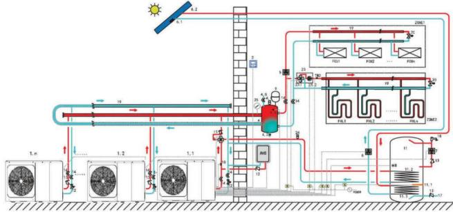
High temperature heat pumps for heating, cooling and domestic hot water production
