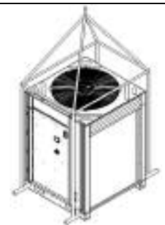
3) Handling by mean of belts N.B. The pipes must have passages pivots or other fasteners to prevent the straps from being released.
