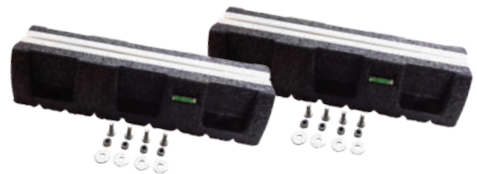
ANTI-VIBRATION FLOOR BASE IN VULCANIZED RUBBER (HEIGHT FROM THE GROUND MM 95) WITH LEVEL AND SCREWS FOR BOOSTER HR 3.0 - 7.8 - 9.0
